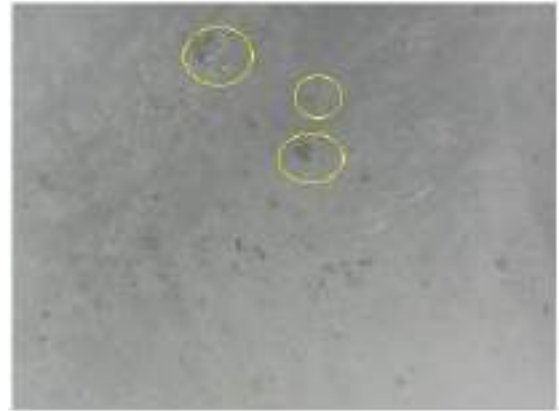
Fig. 6: The formed porosity into microstructure of the alloy at 840 °C, 50x.
