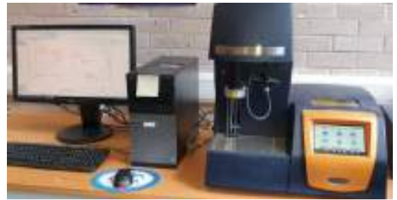
Fig.5: Thermogravimetric (TG) and derivative thermogravimetric (DTG) analyser used in this study (TGA55).
