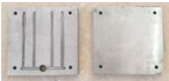
Fig. 1: Fluidity test mould
