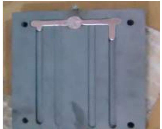
Fig. 2: Photographic view of strip fluidity test casting
