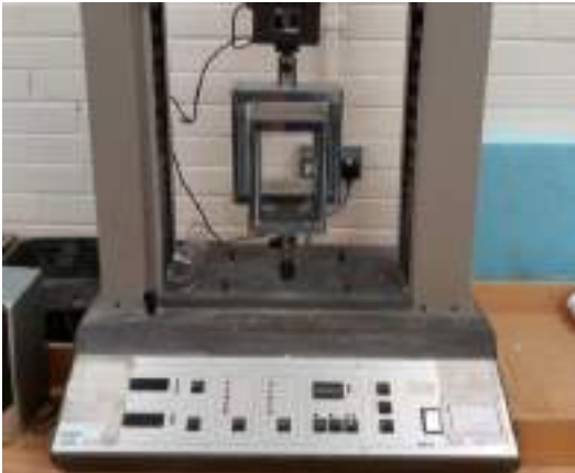
Fig.2: The 10kN capacity Hounsfield compression machine.
