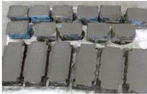
Fig. 2: Compression and flexural test specimen.
