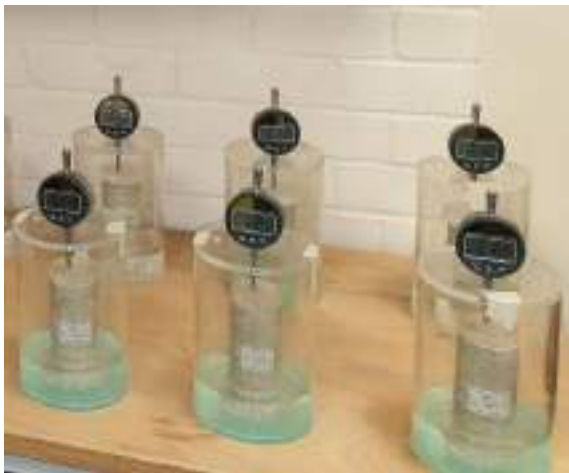
Fig.4: Linear expansion specimens under expansion measurement.
