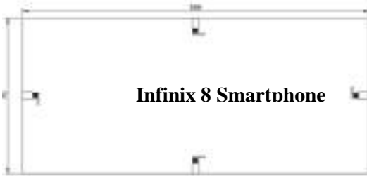
Fig. 13. Layout of the multi port MIMO antenna of CRLH MIMO antenna.
