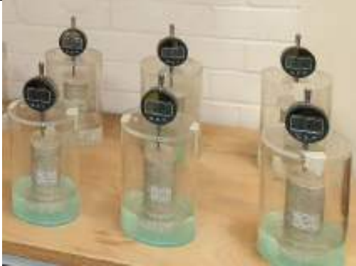
Fig.4: Linear expansion specimens under expansion measurement.
