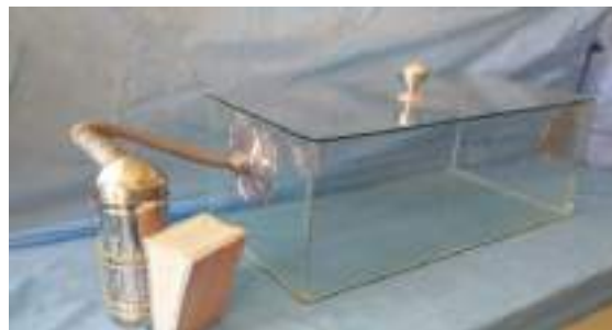
Fig. 1: The smoke-exposure system.
