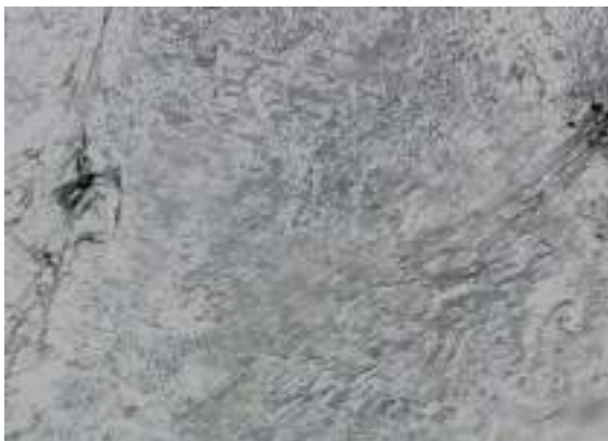
Fig. 4: Segregation process at surface of alloy poured at 800 °C, x50
