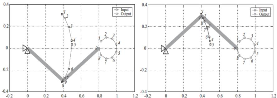
Figure 4: Configuration transitions problems: Newton-Raphson (left); Levenberg-Marquardt (right)
