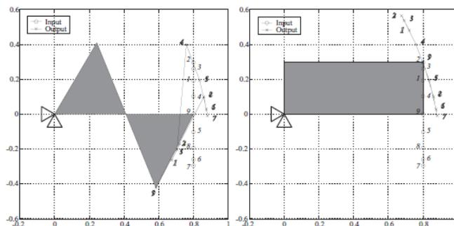
Figure 2: Element distortion problems: Newton-Raphson (left); Levenberg-Marquardt (right)
