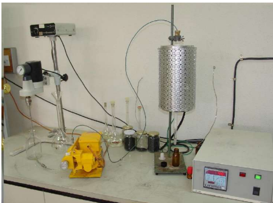
Figure 1: photograph of assembled apparatus used for adsorption.
