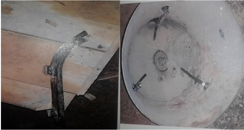
Figure 4: fixing the mixing blades
