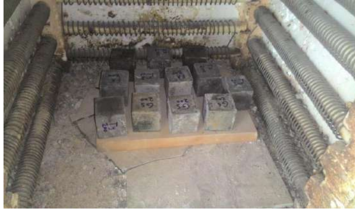
Fig 1: Samples placed inside the electrical furnace after heating
