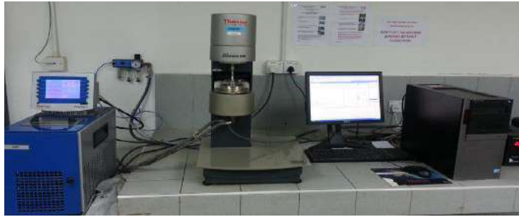
Fig. 4: DSR Equipment and Its Components
