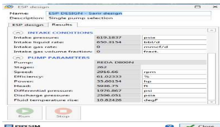
Fig. 12: Well C-349H-65 ESP design parameters obtained using software simulation
